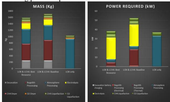
Figure 3: ISRU system hardware comparison in terms of mass (left) and power (right) for each subsystem.
